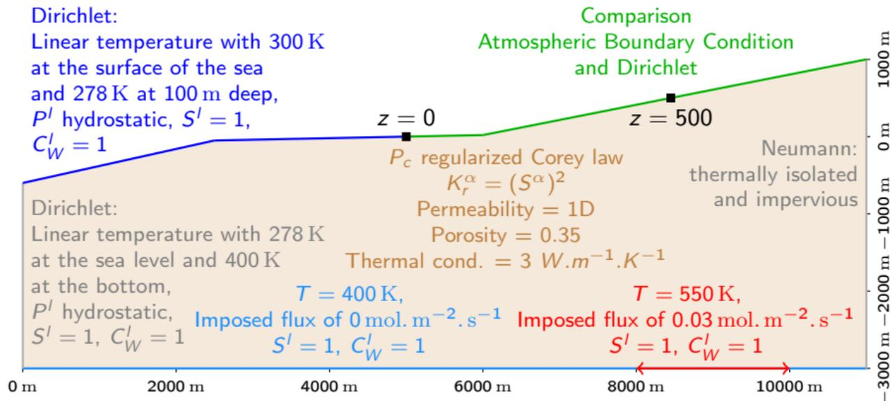
Liquid density and viscosity are fixed to prevent thermal instabilities.
