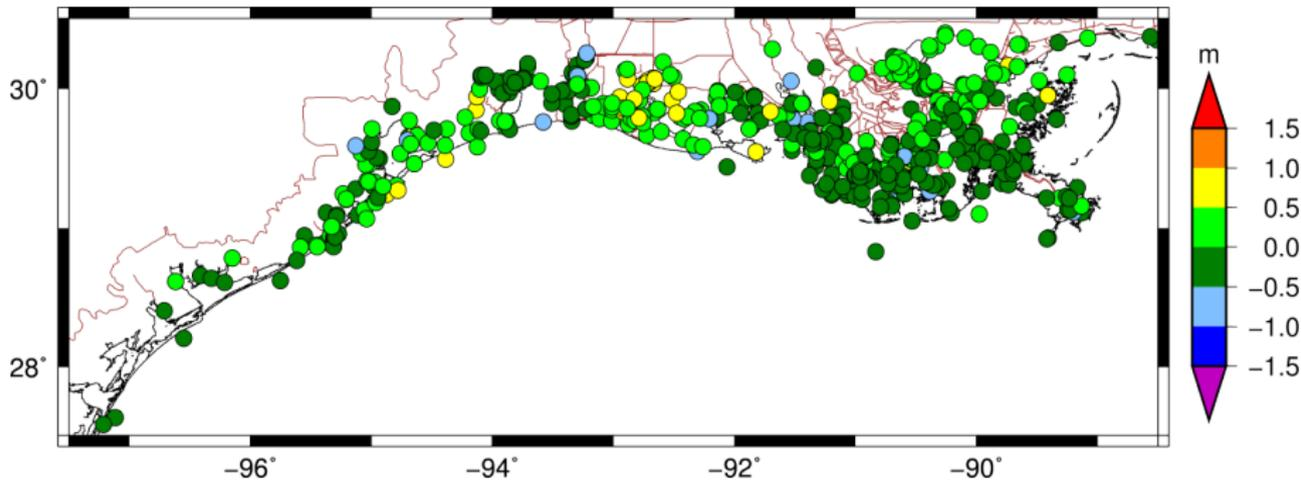
Modeled peak surge vs. measurements. Green and light green indicate error within  $\pm .5$  meter
