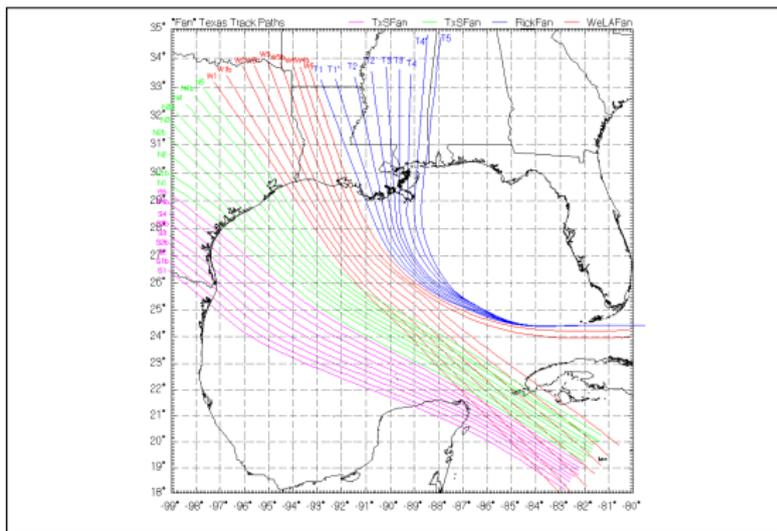
Figure 89: Tracks used to define the synthetic storms. Hurricane parameters vary along the tracks and provide the input to the OceanWeather, Inc., PBL wind/pressure field model. This provides the storm forcing required for each production system simulation.
