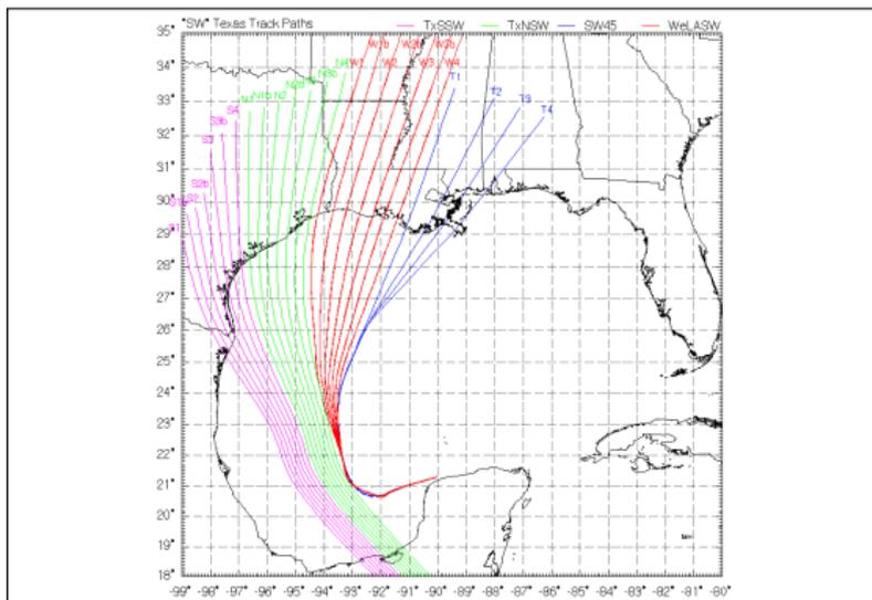
Figure S7: Tracks used to define the synthetic storms. Hurricane parameters vary along the tracks and provide the input to the OceanWeather, Inc., PBL wind/pressure field model. This provides the storm forcing required for each production system simulation.
