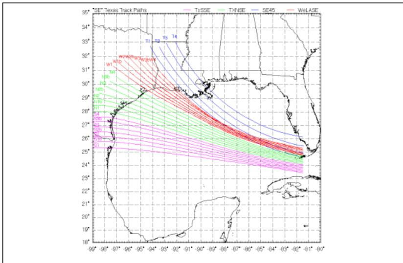
Figure 88: Tracks used to define the synthetic storms. Hurricane parameters vary along the tracks and provide the input to the OceanWeather, Inc., PBL wind/pressure field model. This provides the storm forcing required for each production system simulation.
