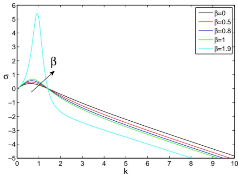
Figure: Plot of growth rate  $\sigma$  versus  $k$  for several values of  $\beta = 4 \langle u^0 \rangle (\lambda_1 - \lambda_2)$ . Collaborator: Gelu Pasa
