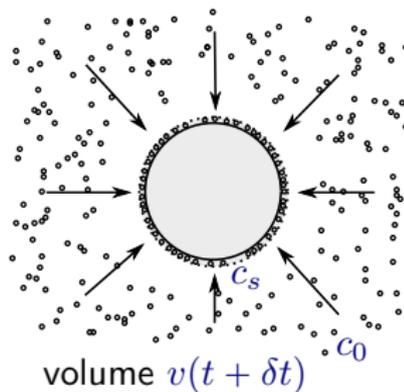
The growth rate of a particle of diameter  $d(t)$  and denoted  $g$  depends on many parameters:
