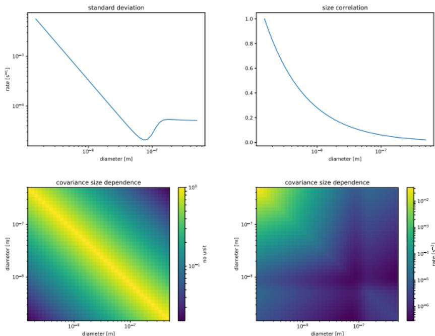
**Figure:** Creation of the covariance matrix of a model. a) size-dependence of the variances, b) correlation, c) Toeplitz matrix of the correlation, and d) covariance matrix of the model.
