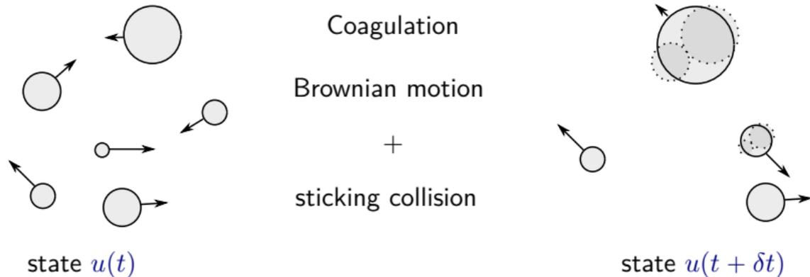
For the Brownian coagulation, the collision frequency factor is given by [FW66]:
