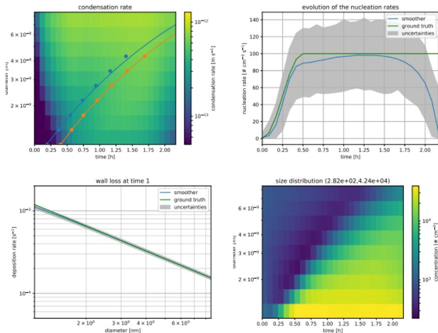
**Figure:** Estimation of the parameter of the GDE for aerosols from a simulated transition to steady state data: 1) growth rate, 2) nucleation rate, 3) loss rate, and 4) number concentration.
