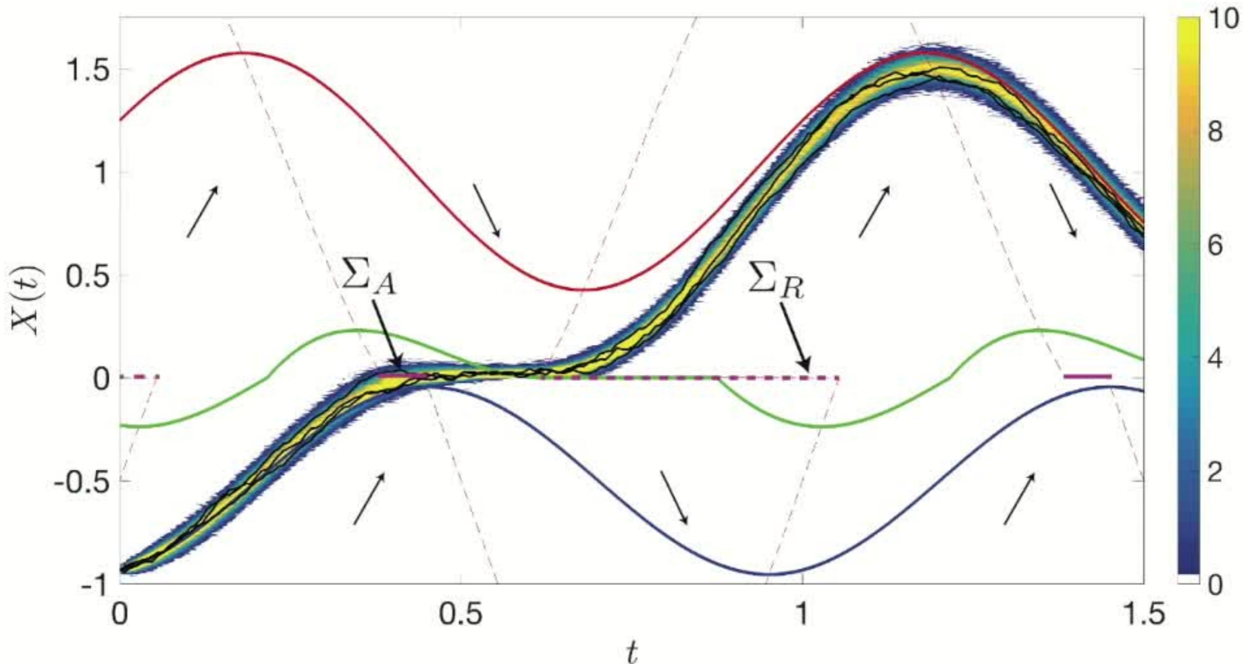
$$dx = \begin{cases} [-r_+(x-1) + A_+ \cos(2\pi t)]dt + \sigma dW & \text{if } x > 0 \\ [-r_-(x-x_0) + A_- \cos(2\pi(t-p))]dt + \sigma dW & \text{if } x < 0 \end{cases}$$
