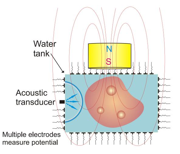
Ultrasound makes electrones and ions vibrate.
