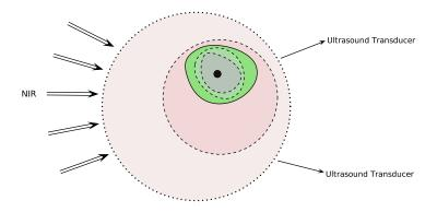
Figure : Photoacoustic Tomography: To recover scattering, absorption and photoacoustic efficiency properties of tissues from boundary measurement of acoustic signal generated with the photoacoustic effect. Two processes: propagation of NIR radiation and propagation of ultrasound. There is a (time) scale separation between the two processes.
