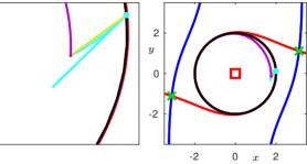
$\blacksquare$  By moving the end point of  $\Gamma$  along the linear approximation, a new trajectory is created.
