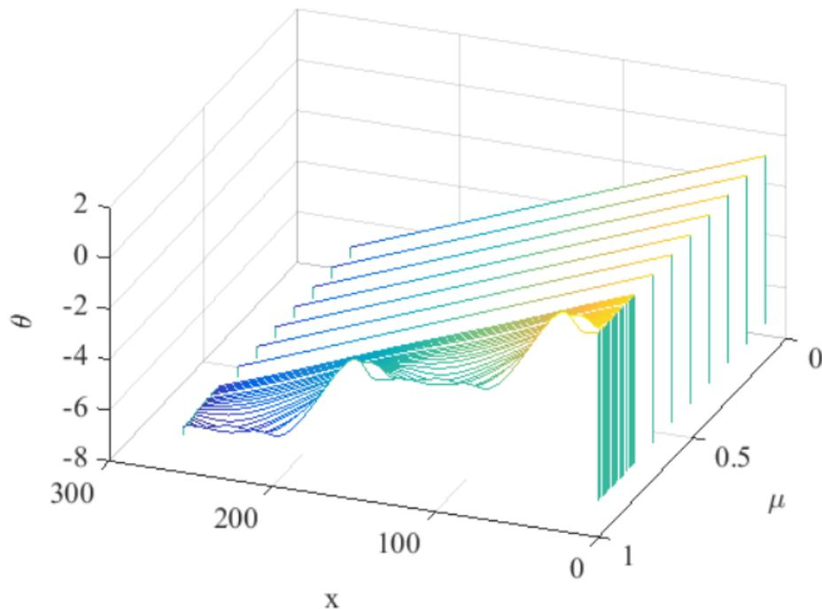
Profile of  $\theta$  on one side of the “jump” as a function of  $x$ , for different values of  $\mu$ .
