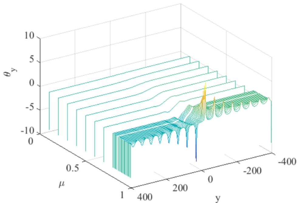
Profile of  $\theta_y$  at  $x = L_x/2$  as a function of  $y$ , for different values of  $\mu$ .
