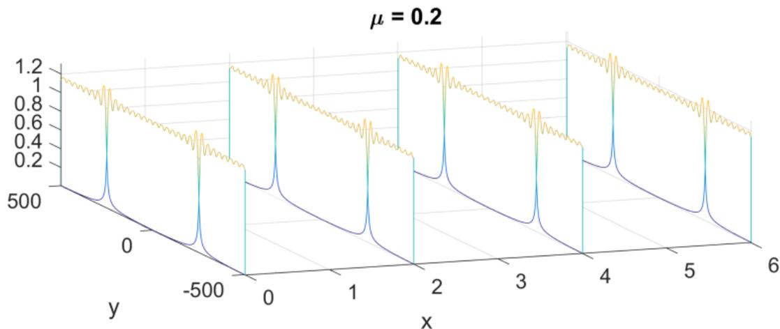
Envelope of both patterns as a function of  $x$  and  $y$ , showing two heteroclinic orbits corresponding to two grain boundaries
