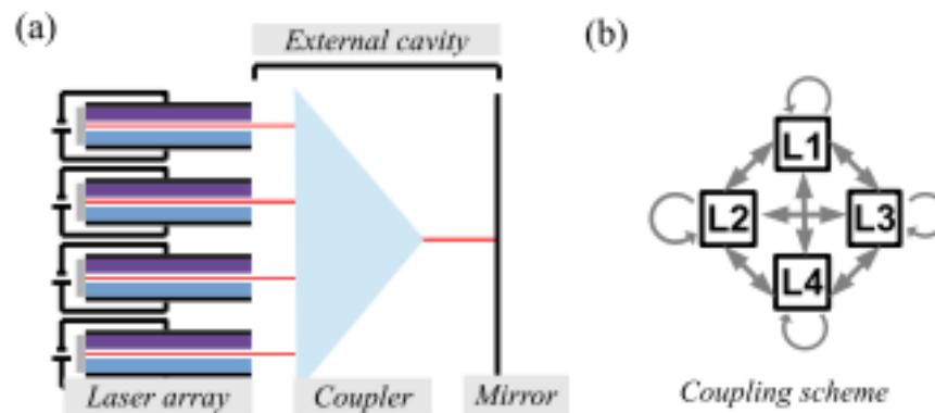
FIG. 1. (Color online) (a) Scheme of a laser array coupled by a common mirror via an external cavity. (b) All-to-all coupling scheme.
