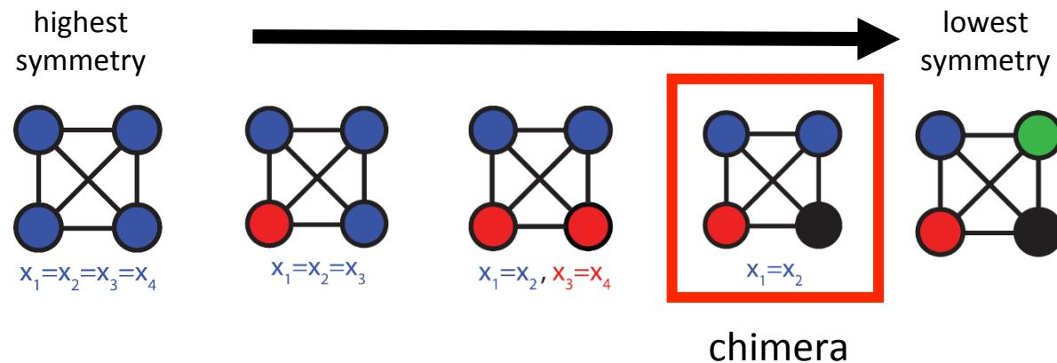
Global coupling: symmetries allow **ANY** combination of nodes to form a cluster.
