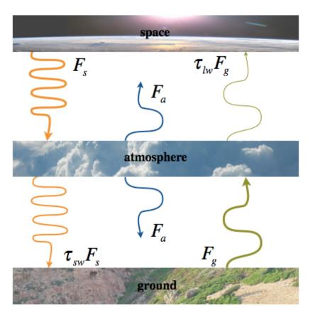
Atmosphere transmits larger fraction of shortwave ( $\tau_{sw} = 0.9$ ) than longwave ( $\tau_{lw} = 0.2$ ) radiation
