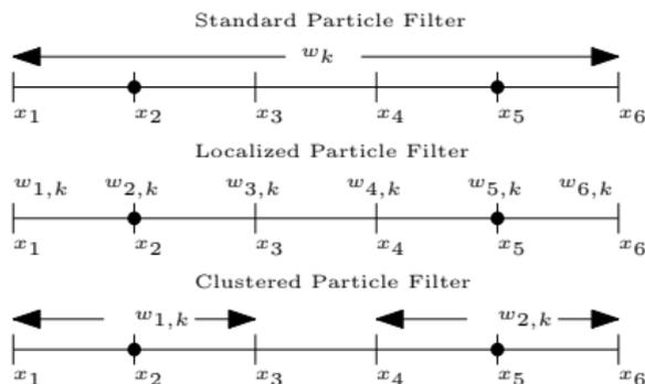
Figure: Schematics of particle weight,  $w_k$ , for the  $k$ -th particle.
