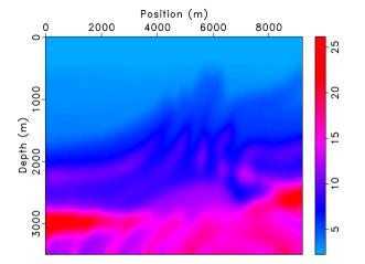
Background bulk modulus map  $\kappa_0$  (density = 1 g/cm<sup>3</sup>) transparent (geometric optics), determines time of travel
