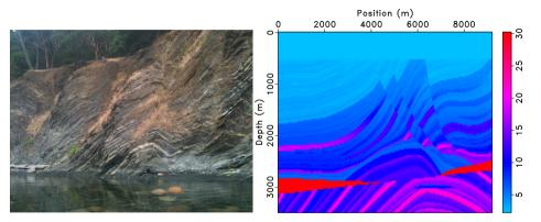
Left: Outcrop, Stuart I., WA (WS, 8/11). Right: Marmousi synthetic model (IFP 89): bulk modulus map  $\kappa$ , unit = GPa (density = 1 g/cm<sup>3</sup>)
