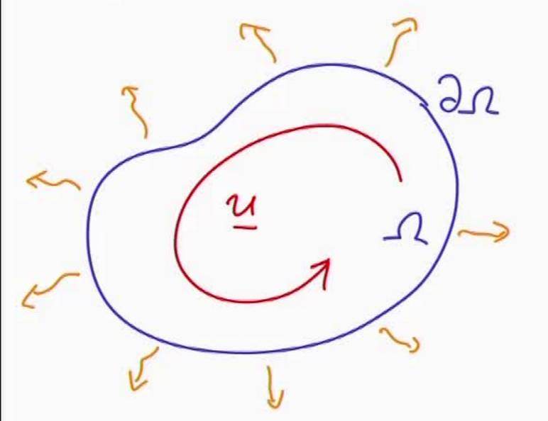
This is the heat exchanger configuration: given an initial distribution of heat, it is fluxed away through the cooled boundaries.
