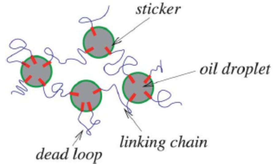
schematic of telechelic polymers
