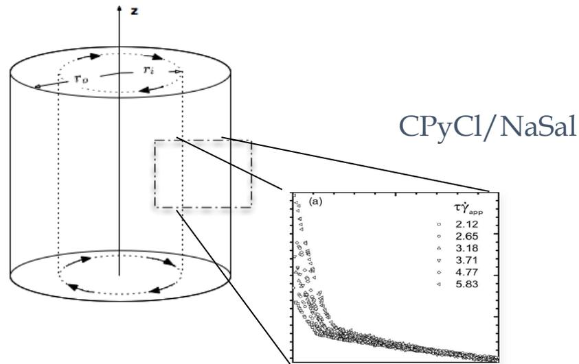
At higher velocities shear bands appear -- a high shear rate band near the inner wall and a low shear rate band near the outer wall
